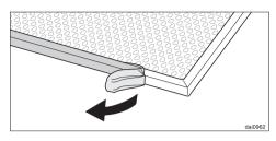
Take out the grease filter and remove the protective foil from the filter frame.
